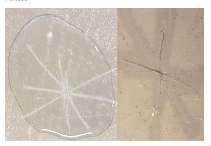
Photo on the left above shows that water is unable to get underneath the lacquer whereas on the right water has clearly been absorbed.
