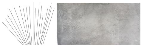
Distribute a thin scraped layer applied in short swirls. Apply 1,2kg of Micro BASE per m2 in a short swirling motion. The thickness of the layer will make the trowel jump and the fringe will appear. (shuttering) Scrape the Micro BASE with the Micro TOP.
